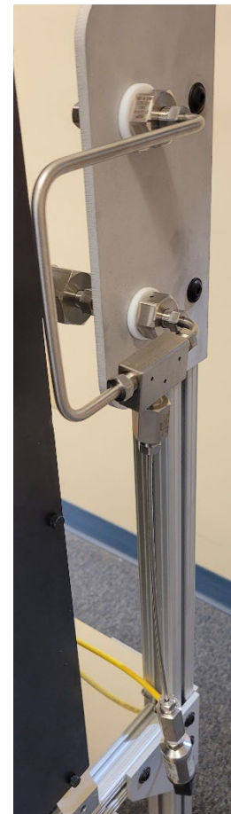
Figure 12: Sensor connected to bulkhead panel
