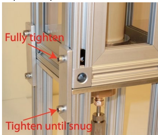
Figure 18: Protective box arm screw tightening scheme
