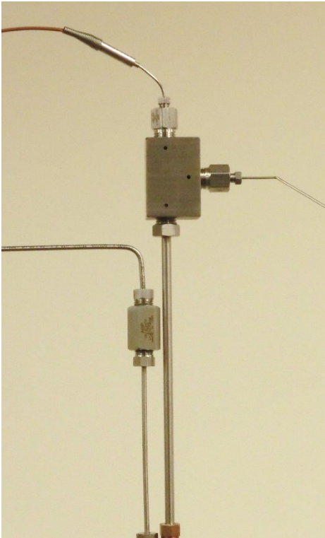
Figure 19: Thermocouple setup for sample temperature monitoring
