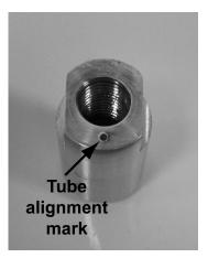
The base component of the cell has been marked with a punch. This mark was made durina certification the process of the cell to reflect the alignment of the tube relative to the base. The center of the serial number on the tube should be aligned with this mark when assembling the cell. This will assure consistent setup.
