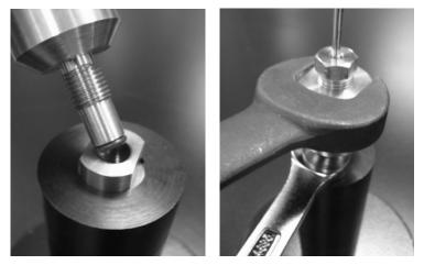
Once the setup of the cell has been completed it should be checked for proper fit in the NMR before pressurizing the sample.
