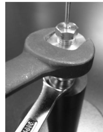
Once the setup of the cell has been completed it should be checked for proper fit in the NMR before pressurizing the sample.
