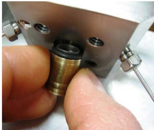
**Figure 18: Reinserting the window plug**
