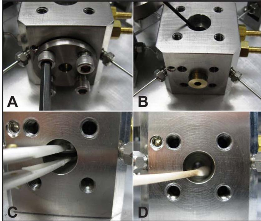
**Figure 16: Replacing the mixing chamber windows**
