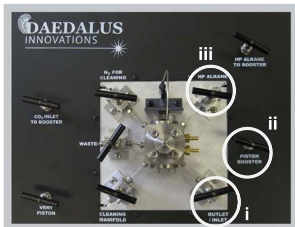
**Figure 14: Progression of valve actuation for the sample transfer steps**
