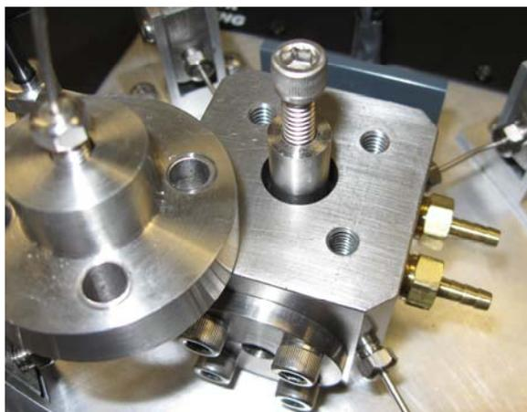
**Figure 15: Removing the piston**
