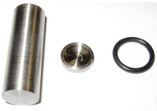
**Figure 10: Mixing chamber components: Piston, reagent plate, and main seal (MCCS).**
