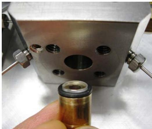
**Figure 17: Reassembly of the window plug**
