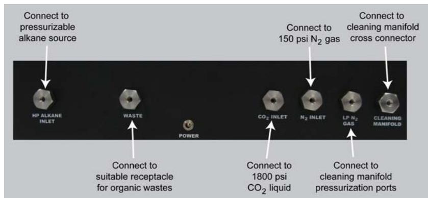
**Figure 8: Back panel port connections**
