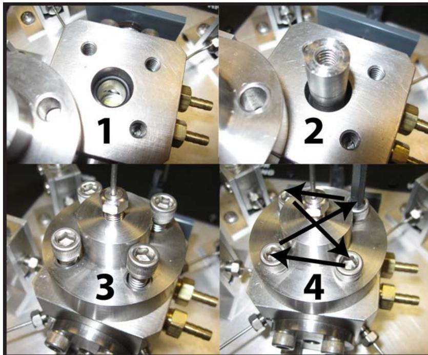
Figure 12: Progression of steps for assembling and sealing the mixing chamber prior to sample preparation
