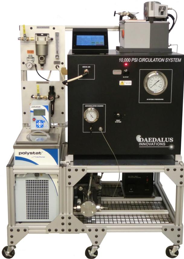
This circulation system has been designed to work directly with all our existing overburden cells for pulseless delivery of fluid up to 10,000 psi, 150°C with operational characteristics that are essential for high quality data collection.
