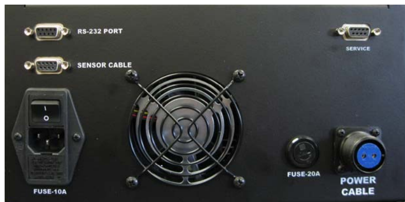
Figure 1: Back of the pump controller box.
