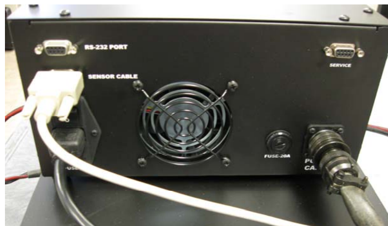
Figure 2: Controller connected for standard operation.
