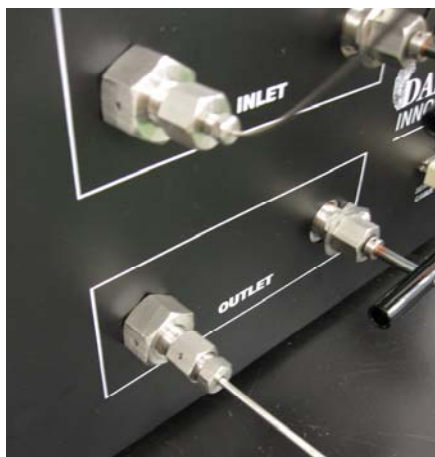
Figure 4: Connecting 1/8" tubing to the outlet port.
