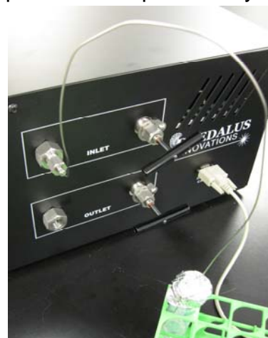
Figure 3: 1/16" tubing used for the fill line connected to the Xtreme-60 inlet port.
