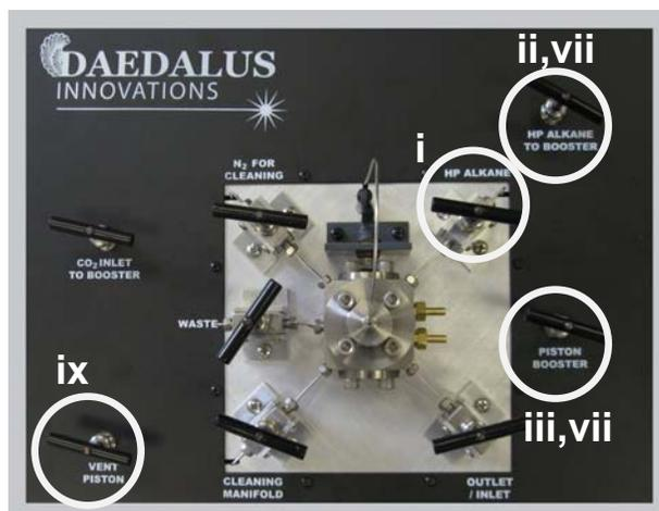
**Figure 13: Increasing the sample chamber pressure using the piston**
