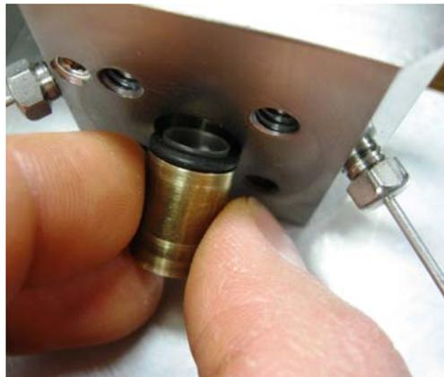
**Figure 18: Reinserting the window plug**
