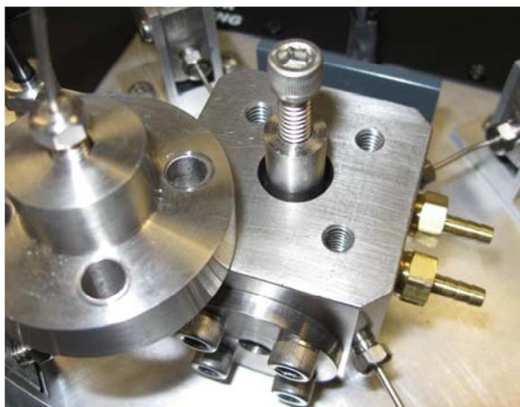
**Figure 15: Removing the piston**
