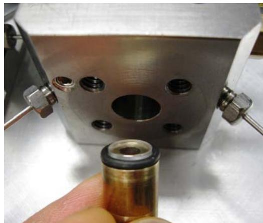
**Figure 17: Reassembly of the window plug**
