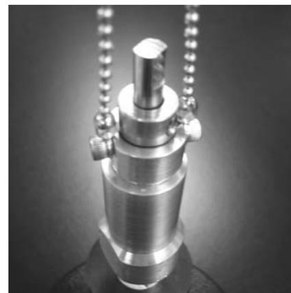
Be sure to keep the pressurized cell inside the protective box when moving the cell. This keeps the user safe as well as minimizes the chance of hitting the tube against objects.
