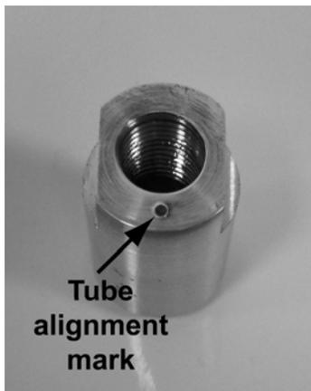
The base component of the cell has been marked with a punch. This mark was made during the certification process of the cell to reflect the alignment of the tube relative to the base. The center of the serial number on the tube should be aligned with this mark when assembling the cell. This will assure consistent setup.
