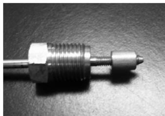
cell. Therefore, be sure the collar is threaded far enough that these two surfaces will meet otherwise the seal integrity could be poor. Once attached this tether should not be removed between uses since repeated disassembly will likely lead to degradation in the sealing performance.
