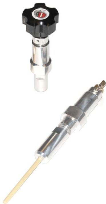
We've taken a high pressure NMR cell and integrated a needle valve into the body to provide a self-contained unit that does not require a continuous connection to an external pressure source. The sample can now be prepared on the bench, the valve closed, and the unit carried to the NMR spectrometer for data collection. Containment of the sample lasts for months without significant pressure loss.
