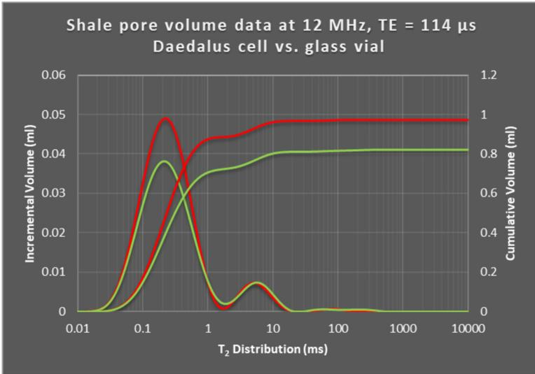
The low background signal from the Daedalus cell allows data to be collected with  $TE = 114 \mu s$ . The green traces are the data of the sample in a glass vial with the red traces the data from the Daedalus cell. Though the Daedalus cell data does show an overestimate of the pore volume the overall agreement is remarkably good. No effort was made to subtract the empty cell spectrum from the sample spectrum in this analysis.
