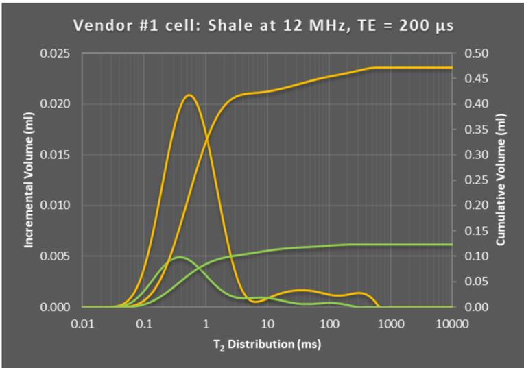
The data from the vendor 1 cell could not be collected with  $TE = 114 \mu s$  due to the background signal overwhelming the sample data signal. The data collected at  $TE = 200 \mu s$  (orange) shows considerable overestimation of the total pore volume. Further, due to the high background signal at low  $T_2$  values the overall fitted trajectory of the trace is influenced such that the overall profile only marginally resembles the glass vial data (green).
